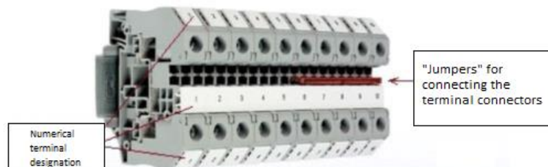
Photo. 6. A method of marking terminal connectors.
