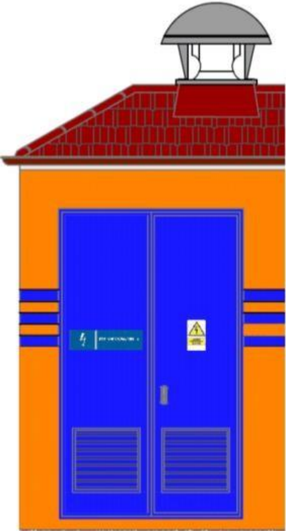
Fig. 22. Information and warning board on transformer chamber door.
